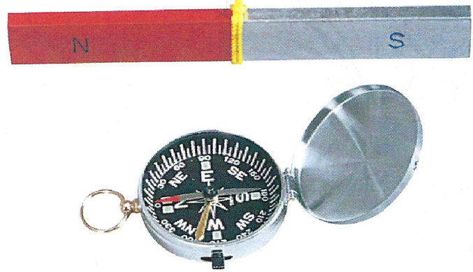
Figure 2 The needle in a compass is a magnet that is free to rotate.
